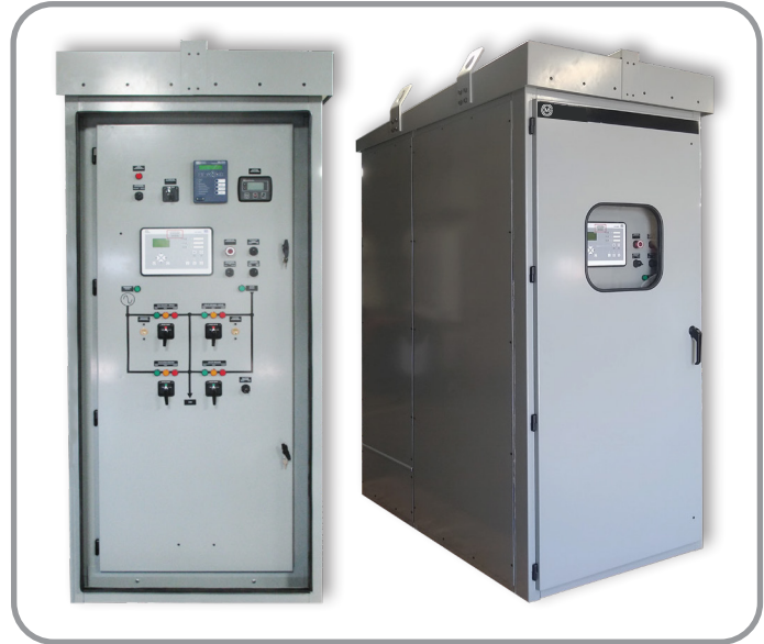
480V, 2000A, bypass isolation ATS, outdoor rated
