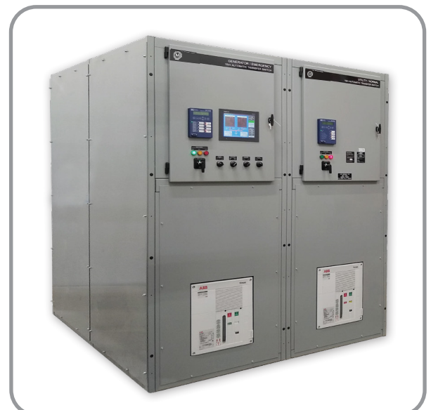
12.47kV, 600A, indoor rated ATS with PLC/HMI-based controls
